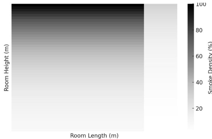
Figure 4c: Smoke Density Distribution with Window Opening.
